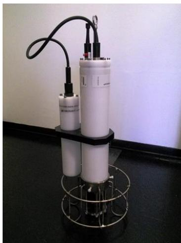
Fig. 2.3 Sonda Idronaut mod. Ocean Seven 316 Plus
