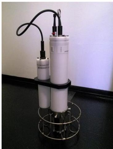
Fig. 2.2 Sonda Idronaut mod. Ocean Seven 316 Plus
